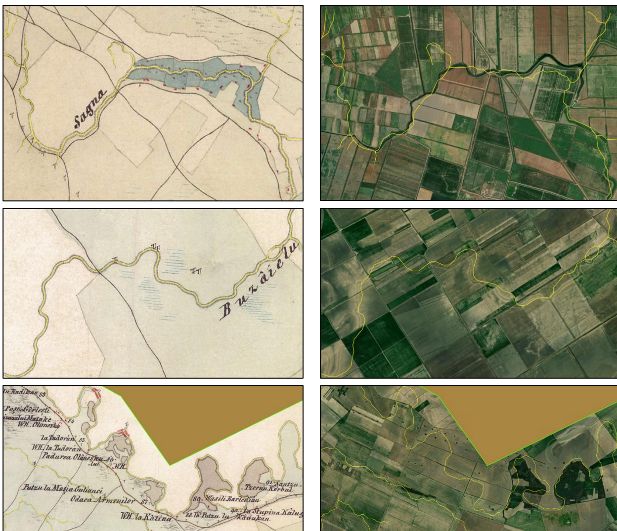
Figure 17. Dry ditches digitising over the historical map in yellow and the same lines over the current optical imagery.
